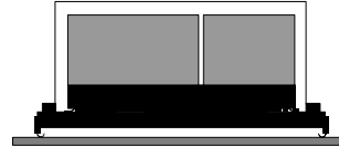
Figure 5: Sectional view of a 640Mbit memory MCM
