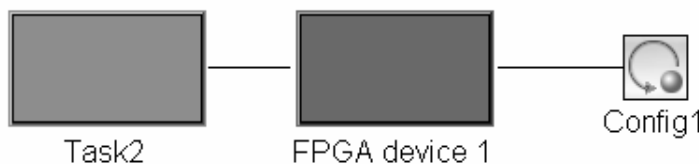
Figure 6: The “Task2” box indicates a task option, the “FPGA device 1” box indicates the target device onto which the task is mapped, and the “Config1” box indicates an operating state
