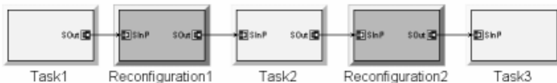
Figure 3: Application modeling. Tasks are the lighter shaded boxes, and state transitions are the darker ones. Dataflow is indicated with directed connections (black arrows).
