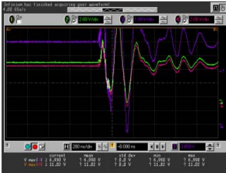
Figure 4 : Spike on Vcca and Vcci in a Burn-in oven
